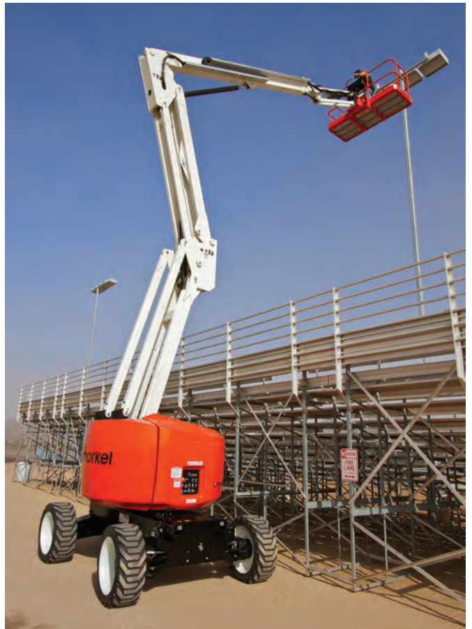
LEFT AND RIGHT: The upgraded version of Snorkel A62JRT articulated boom lift has entered full production. The machine is capable of lifting up to 227 kg, with a maximum working height of 20.8 m.
