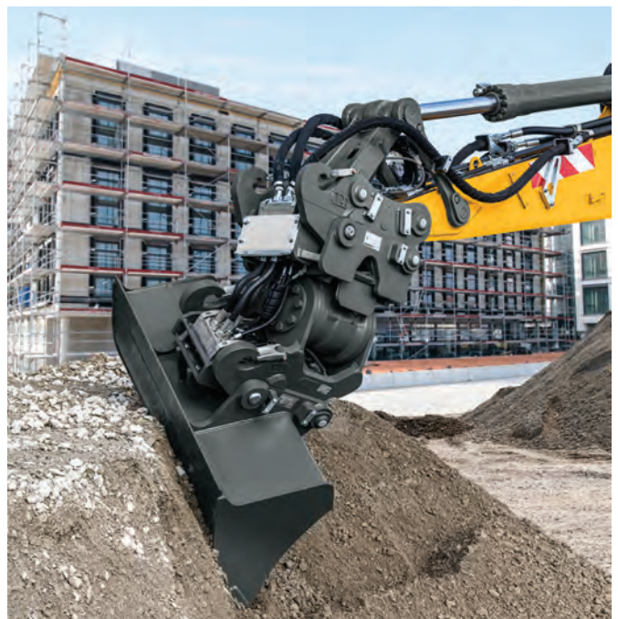
BELOW: As a sandwich attachment, the connection between stick end and LiTiU, as well as the bottom of the LiTiU and attachment, is realised with a fully automatic quick coupling system. This allows swing angles of up to 2 x 50°.
