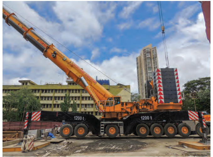
ABOVE: The AC 1000-9 has a 1,200-t capacity. In this project, the crane had to be equipped with its full 228-t counterweight for a boom length of 30 m.
