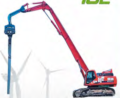
Excavator Vibro Hammer
