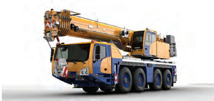
ALL IMAGES: The new AC 80-4 all terrain crane features a compact design, offering a maximum main boom length of 60 m.
