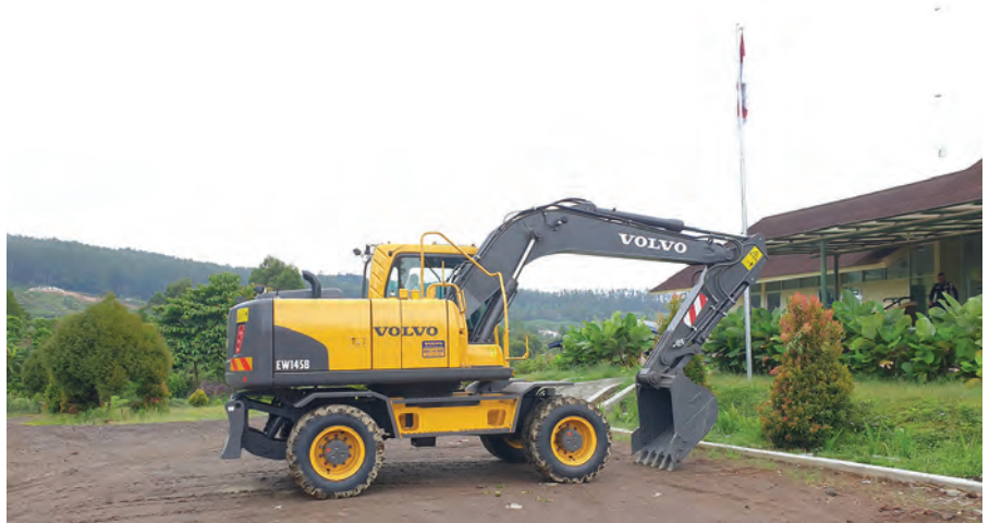
TOP AND ABOVE: Volvo EW145B Prime wheeled excavator features a strengthened undercarriage frame, reinforced boom and arm, and long wear components to withstand tough shifts. The machine has been working on the project since May 2019, operating eight hours a day.
