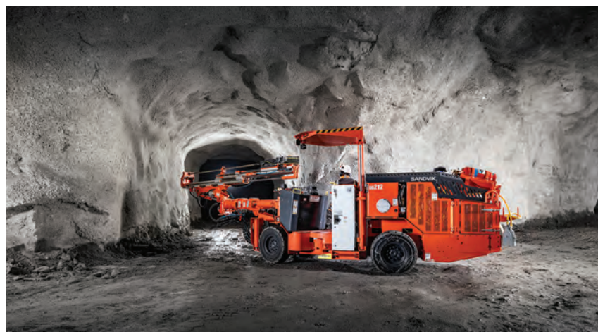
Sandvik DD212 drill rig is equipped with an intelligent boom.
