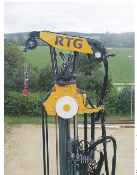
BELOW RIGHT: The new auxiliary winch for RG telescopic leaders.
